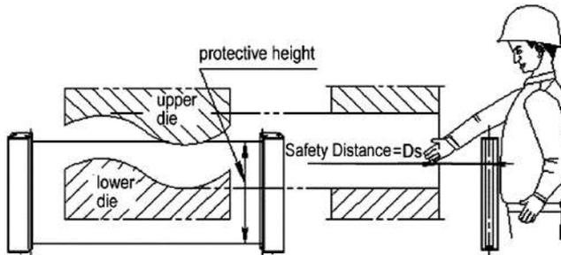
Fig2.1.4 Incorrect position of installation site
