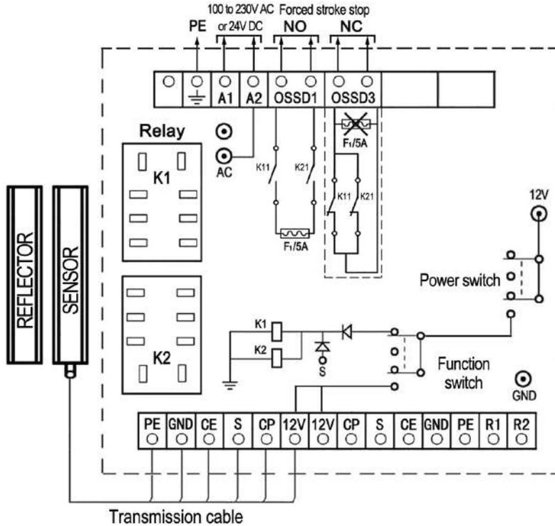
Fig3.4 CQ1 type controller wiring
