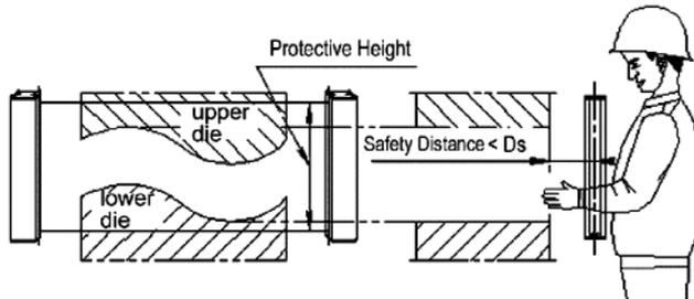
Fig2.1.2 Incorrect position of installation site
