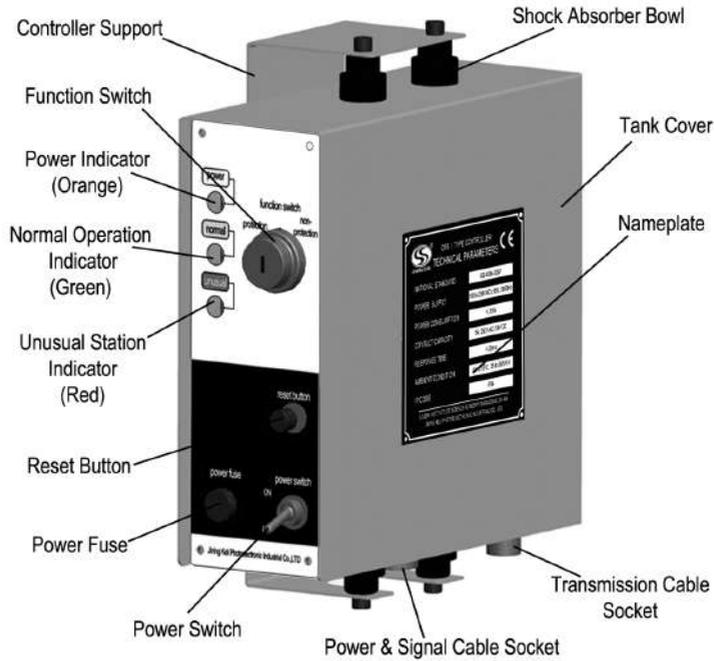
Fig1.2.A CPS I type controller–Single–side protection
