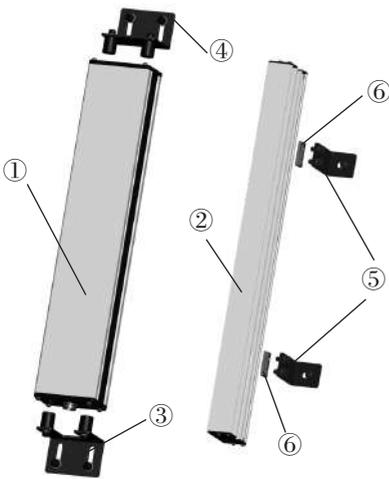
Fig2.4 Common side mounting (PC)
