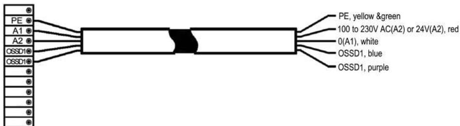
Fig1.5.B Power & signal cable for CQ1 type controller
