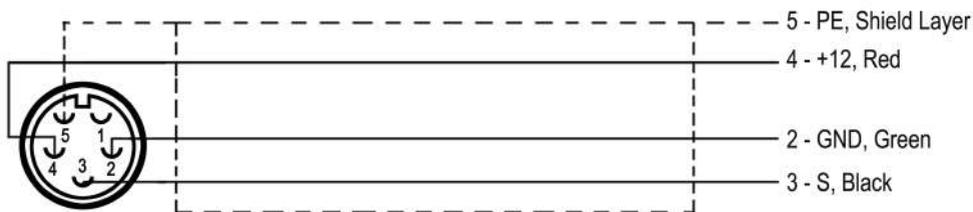
Fig1.4.B Transmission cable for CQ1 type controller
