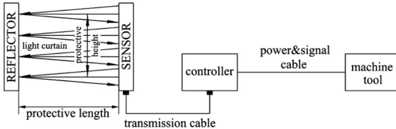
Fig1.1 Schematic illustration of working principle
