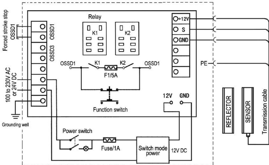
Fig3.1.A CPS I type controller wiring – Single-side protection
