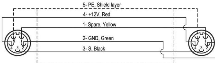
Fig1.4.A Transmission cable for CPS I type controller
