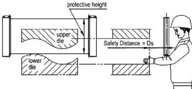
Fig2.1.3 Incorrect position of installation site
