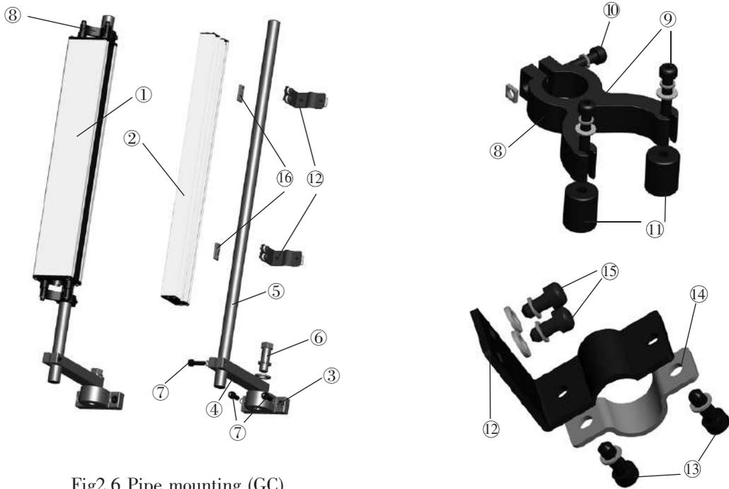
Fig2.6 Pipe mounting (GC)
