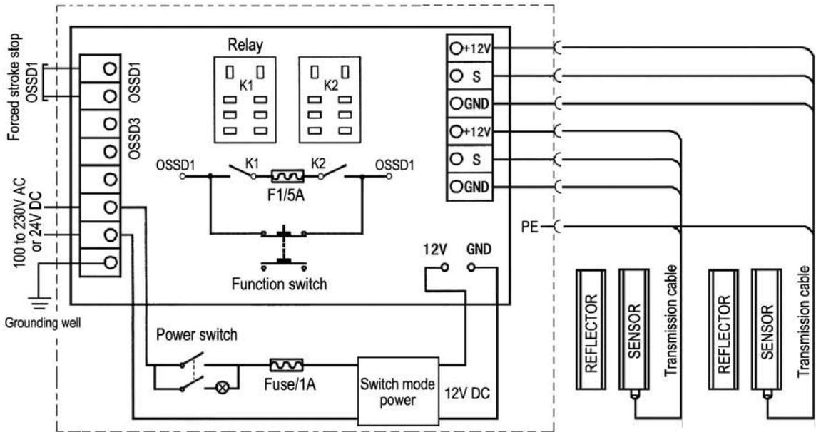
Fig3.1.B CPS I type controller wiring – Double-side protection
