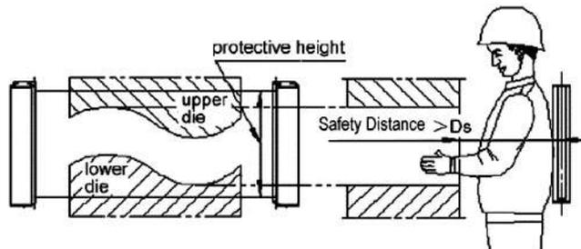
Fig2.1.5 Incorrect position of installation site
