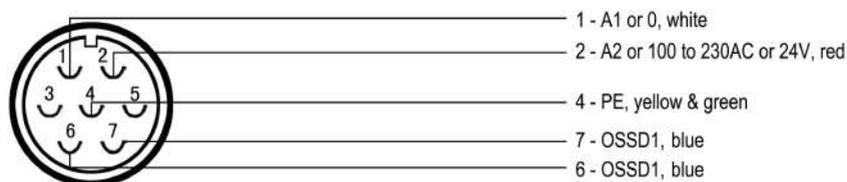
Fig1.5.A Power & signal cable for CPS I type controller
