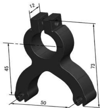
LDKS pipe-mounting fixing clamp
