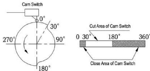
Fig4.1 Structure & Functional mode of cam switch
