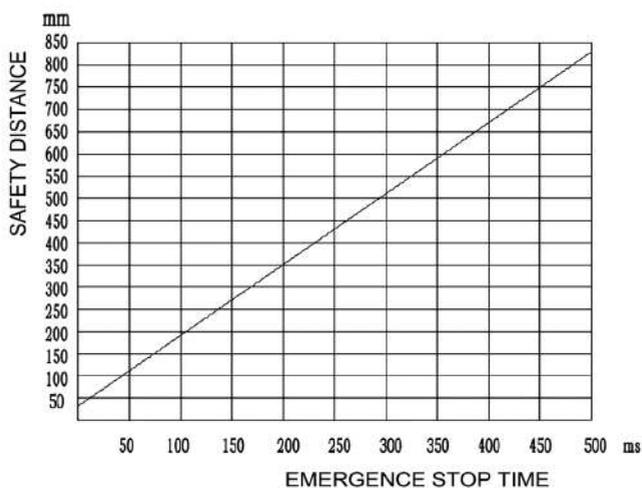
Sheet2.1 Calculation sheet for safety distance
