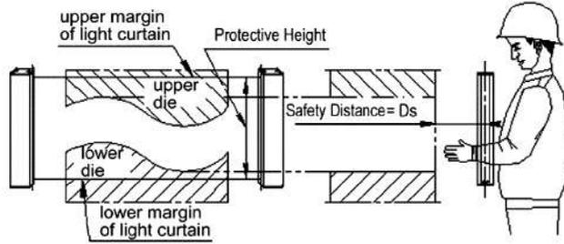
Fig2.1.1 The correct position of installation site
